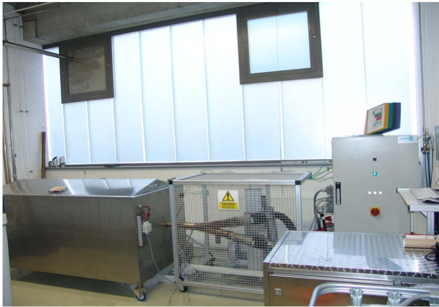
Figure 3.16: Overview of a constructed corrosion rig
