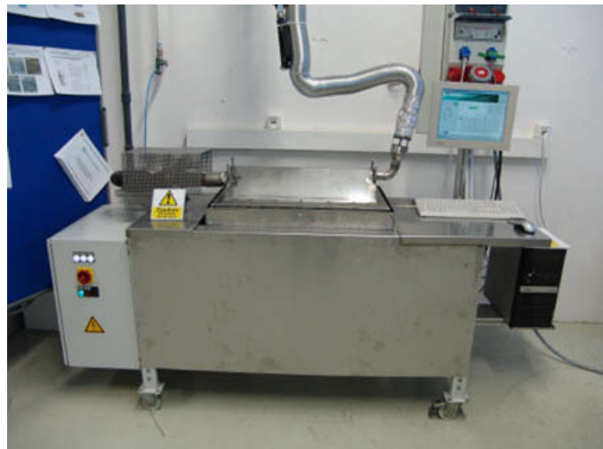
Figure 3.12: Overview of a constructed dip and dry testing equipment
