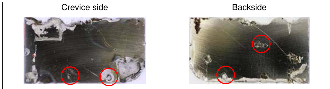
Figure 4.35: 1.4509 specimen surfaces after measurement in 6% \text{FeCl}_3 – 0.1 mm crevice
