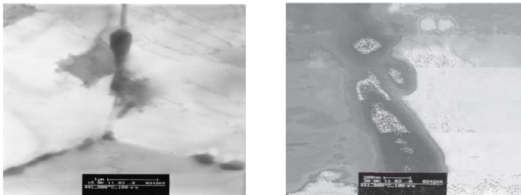
Figure 4.11: TEM micrograph 1.4509 treated 100h at 800°C
