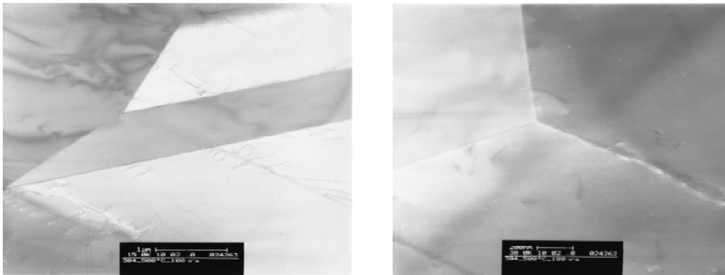
Figure 4.15: TEM micrograph 1.4301 treated 100h at 500°C
