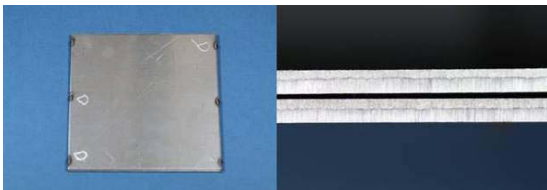
Figure 3.7: Specimen assembly with well defined crevice
