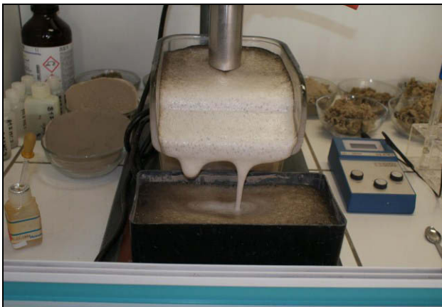
Figure C3-3: Flotation occurs after adding Flotanol D12 as a frother – froth product collected in a tab.
