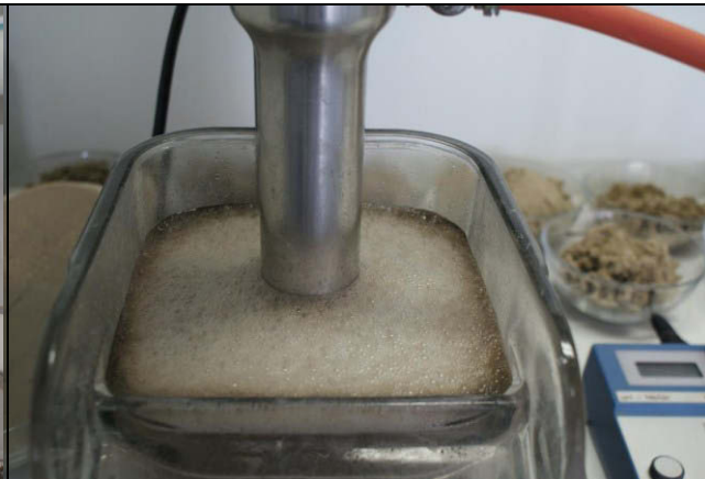
Figure C3-2: Hg-Sulfid floated to the surface (KAX as collecting agent)
