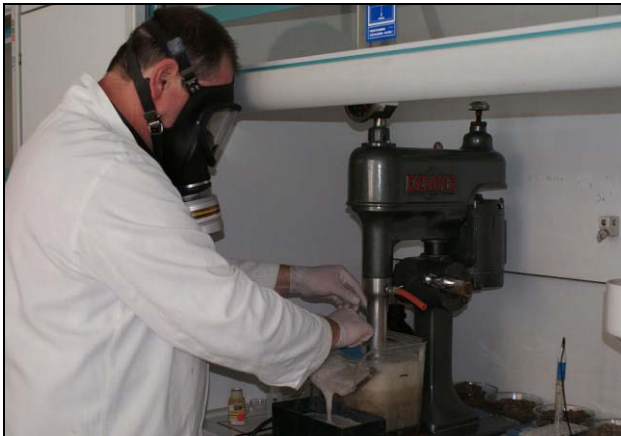
Figure C3-1: Flotation of Hg-contaminated soil, test rows performed with 800, 1000 and 1200 [mg/kg]
