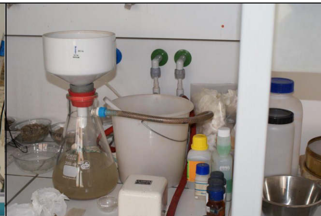
Figure C3-4: Suction strainer supported by a water-jet vacuum pump for dewatering of the froth product
