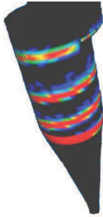
Figure 50: CFD erosion 250 mm cyclone old head
