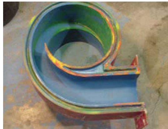
Figure 45: Wear/paint test new inlet
