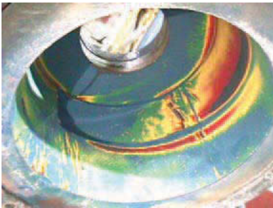
Figure 46: Wear/paint test standard inlet
