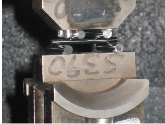
Fig. 23: Four point bending test setup with inner and outer span length of 15 and 30 mm
