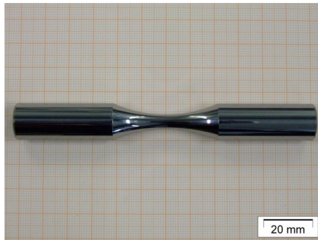
Fig. 8: Specimen geometry S1 (Hourglass-shaped specimen, minimum diameter = 6 mm) tested in uniaxial tension and compression tests
