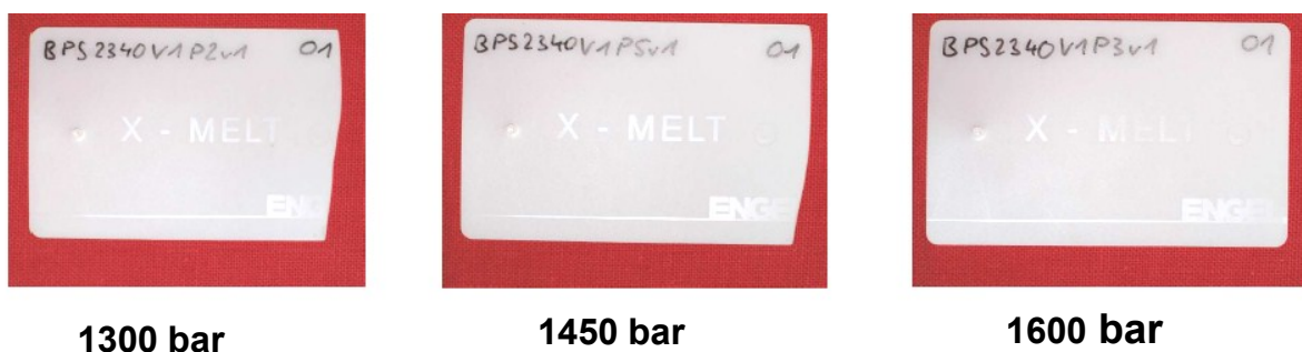
Figure 119: Photos of the produced check-card parts at different compression pressures.
