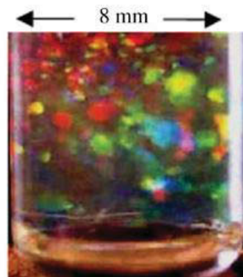
Fig. 2.35. Iridescence from a 3D colloidal PhC with bcc lattice consisting of silica spheres dispersed in ethylene glycol-water mixture under white light illumination. The color spots correspond to single-crystalline domains. Taken from [102]
