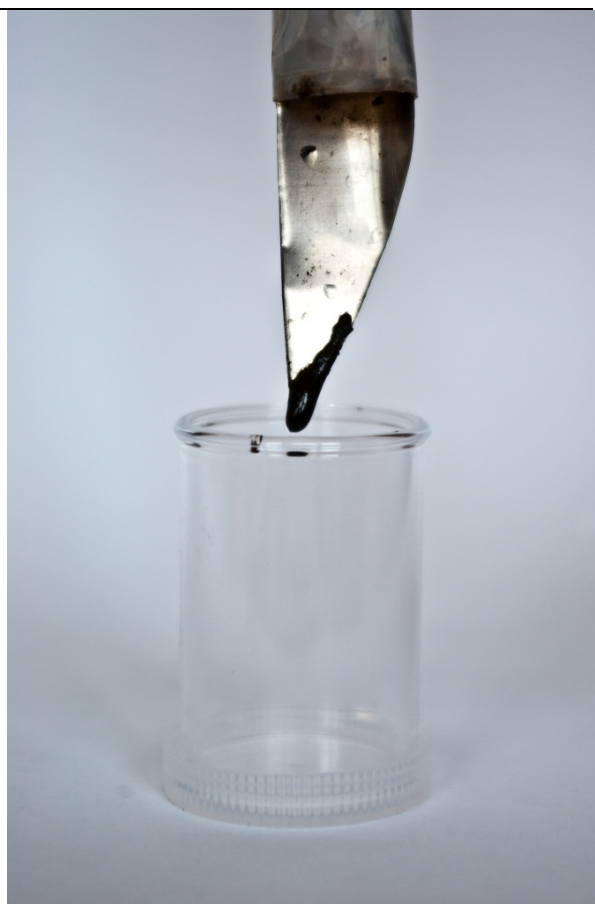
b- Extraction of magnetic material with \mu -metal needle
