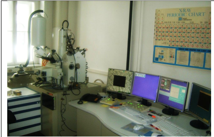
Electron micro probe analyser (EMPA) JEOL JXA 8200
