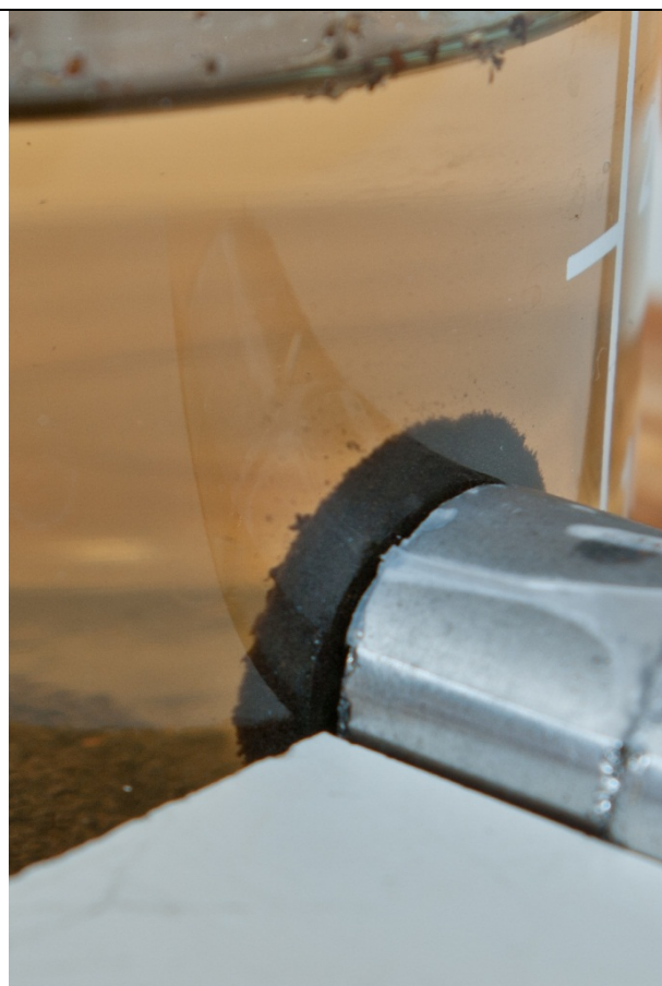
a- Concentrate of magnetic material with hand magnet, after dissolving soil in milli-Q water
