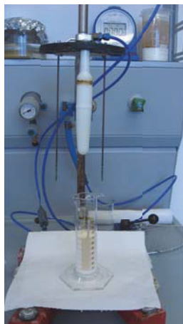
Fig. 25: Porcelain former that is used for thin XNBR film formation by coagulation.
