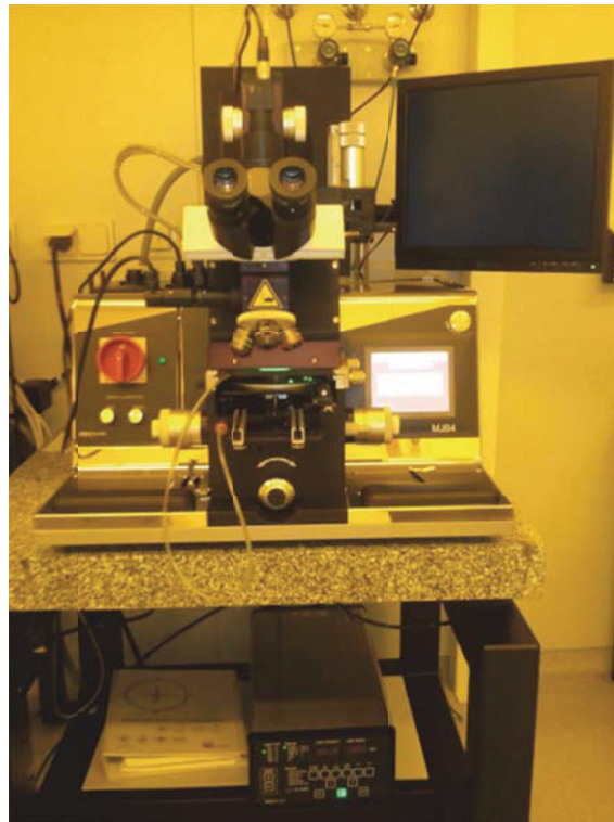
Fig. 9: Süss MJB4 Mask Aligner, which was used for photolithographic patterning experiments (© Technical University of Braunschweig, Germany).
