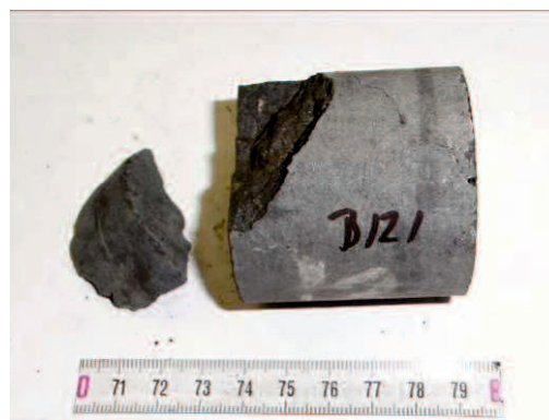
Figure 6-3: Surface part of sample B121 of Weitendorf basalt spalls off after 120 s of irradiation.
