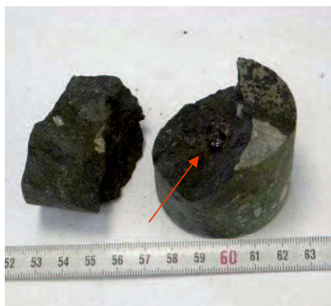
Figure 6-29: Formation of a small spot of melt in the centre of a diabase sample (highlighted by red arrow) of Jakomini quarry after irradiation with microwaves for 120 s..
