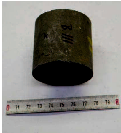
Figure 6-1: Untreated sample of Weitendorf basalt. No cracking visible.
