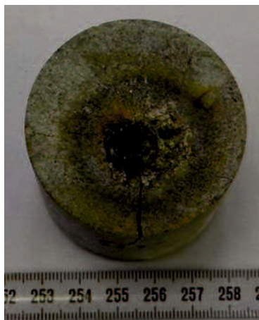
Figure 6-55: Sample SS55 after 120 s of irradiation with additional steel cone. Spallation and melting of material at the surface leading to the development of cracks.
