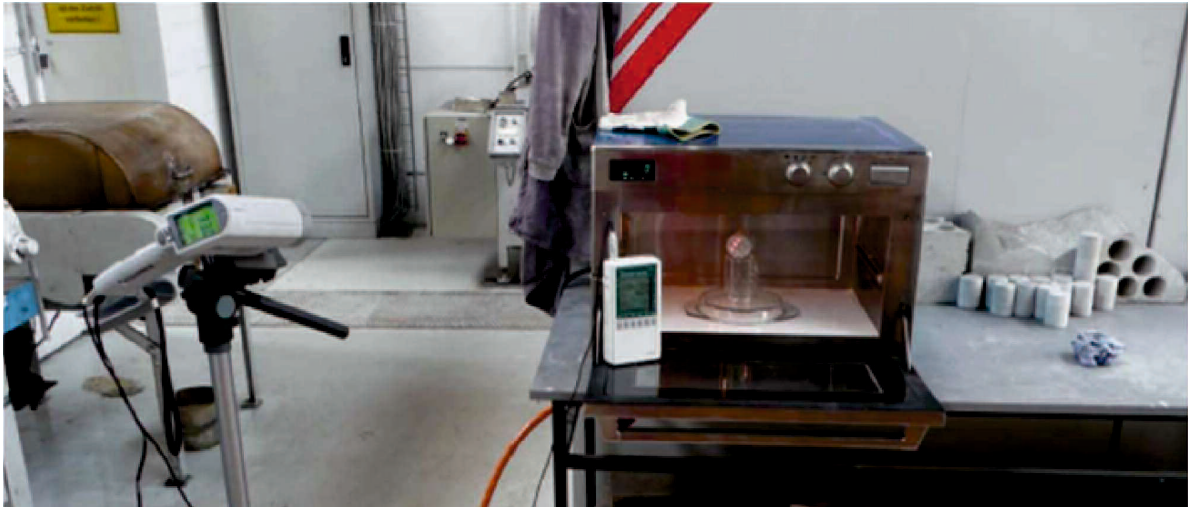
Figure 5-3: Experimental arrangement for small scale laboratory tests. Sample placed in centre of microwave on top of glass cylinder and infrared thermometer with data logger (left and on top of microwave door) for the investigation of surface temperature after irradiation (Foto taken by T. Peinsitt).
