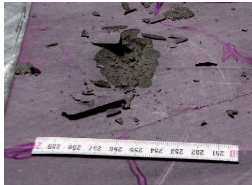
Figure 7-10: Basalt sample after 5 pulses (2s – 20% of 30 kW and 1s – 100% → totally 15 s).
