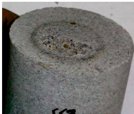
Figure 6-54: Sandstone sample SS3 after 60 s of irradiation with additional steel cone. Significant spallation visible at the surface.
