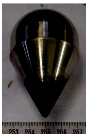
Figure 6-61: After the treatment of Neves Corvo copper ore an unspecified black powder precipitates at the tip of the steel cone.
