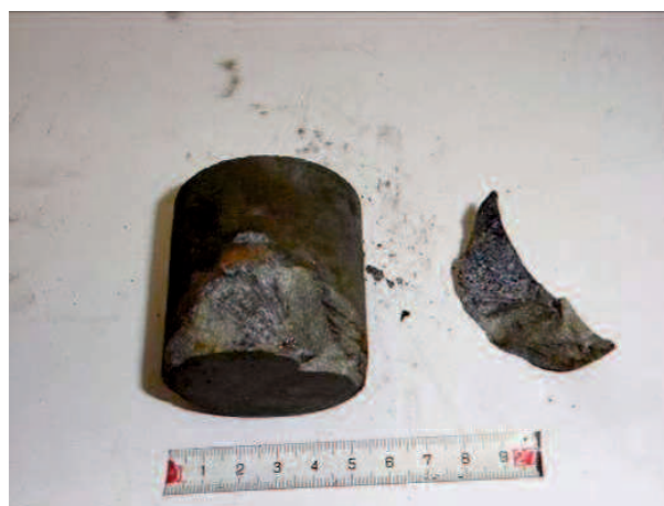
Figure 6-46: Neves Corvo sample after 120 s of irradiation. Ablation of small pieces after microwave irradiation with 3.2 kW.
