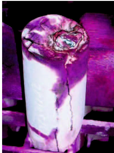
Figure 7-6: Drill core taken from basalt sample after 50 s of irradiation with 25 kW treated with dye-penetrant. One axial crack has a length of approximately 10 cm.
