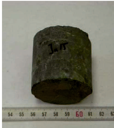
Figure 6-26: Sample Ja15 of Jakomini diabase after 90 s of irradiation. No damage visible.
