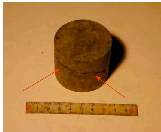
Figure 6-43: Sample Ga09 (gabbro) after 90 s of irradiation with 3.2 kW. A significant circumferential crack is visible (red arrows).
