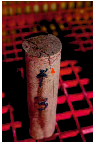
Figure 7-30: Drill core of gabbro sample under spot irradiated for 30 s with 25 kW. Circumferential cracks below the surface (red arrow) and radial crack at surface clearly visible.
