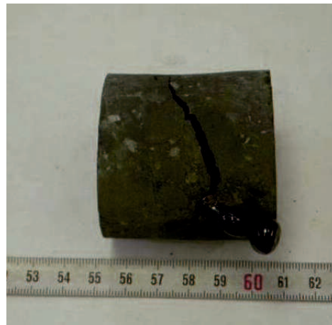
Figure 6-27: Sample Ja13 of Jakomini diabase after 90 s of irradiation. Sample is melting in the centre and subsequent cracking occurs.
