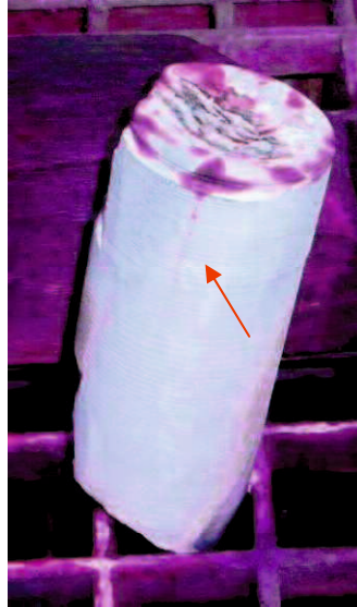
Figure 7-2: Drillcore of basalt sample irradiated for 6 s with 25 kW. One crack developed in axial direction for a depth of approximately 50 mm (highlighted by red arrow).
