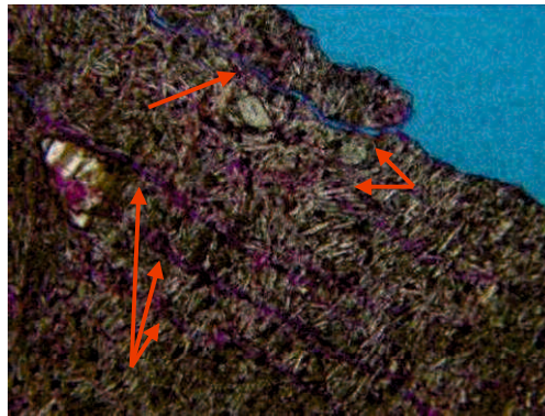
Figure 7-9: Resin saturated thin section of basalt sample after irradiation for 6 s with 25 kW. Fine network of cracks below the surface of spallation area. Cracks indicated with red arrows. Width of picture = 2.9 mm.
