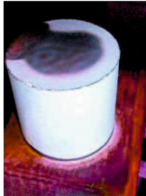
Figure 6-11: Unirradiated basalt sample treated with a dye-penetrant; no visible cracks.
