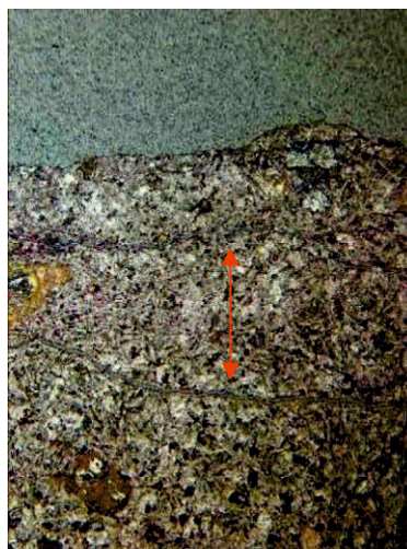
Figure 7-11: Resin saturated thin section of the area beneath the spot shown in Figure 7-10. Cracks (blue and indicated by red arrows) are aligned parallel to main damage patterns and show no affiliation to mineralogical boundaries. Height of picture = 2.9 mm.
