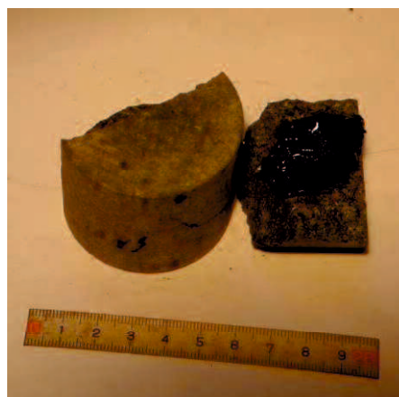
Figure 6-44: Gabbro sample Ga09 after 2 nd irradiation for 90 s resulting in formation of melt and complete disintegration.
