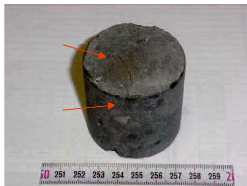
Figure 6-34: Minor cracks in diabase sample Ja25 after the first irradiation with microwaves or 90 s (Cracks marked with red arrows).
