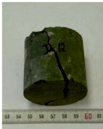
Figure 6-28: Sample Ja12 of Jakomini diabase after 120 s of irradiation. Strong cracking and formation of melt observable.
