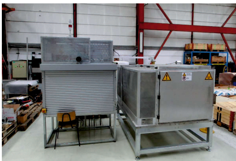
Figure 5-5: Final assembly of microwave test-rig. Magnetron and control unit (covered with a construction of sheet metal; left side) and safety cavity (right side).
