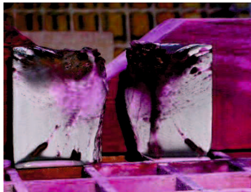
Figure 7-7: Crosscut through a drill core taken from large block of basalt sample irradiated for 50 s with 25 kW. Depth of crack network approximately 45 mm.
