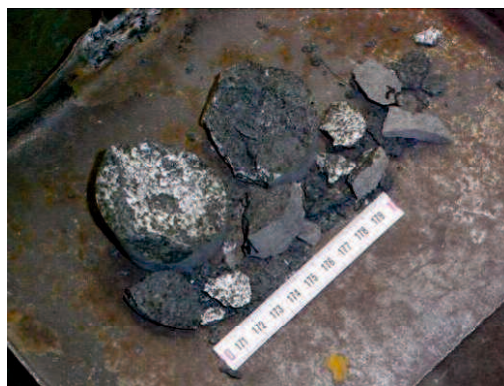
Figure 6-19: Fragments of Klöch basalt shattered after 30 s of irradiation.
