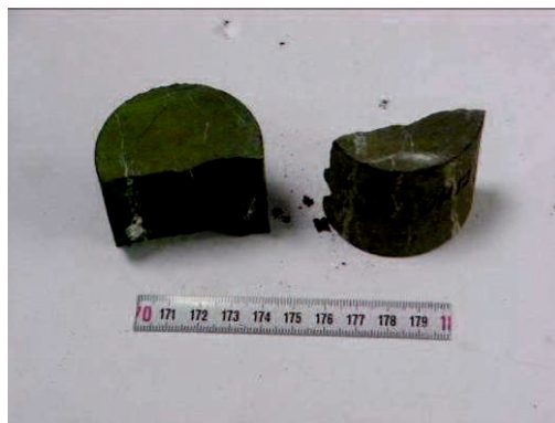
Figure 6-25: Pieces of sample OH12 of Oberhaag diabase which shatters after irradiation for 160 s.
