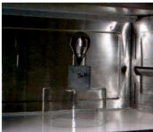
Figure 5-4: Arrangement of steel cone in microwave oven. Glass cylinder, sample and steel cone (bottom to top) inside the cavity. The steel cone is kept in position with help of a glass tube. For the glass parts non-absorbing quartz glass is used.
