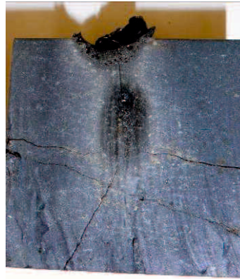
Figure 6-52: Crosscut through basalt sample Ba60 after 120s of irradiation with the help of a steel cone. Molten spot at surface and large cracks throughout the entire sample visible.
