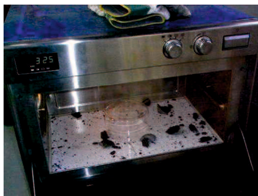
Figure 6-20: Klöch basalt explodes after 30 s of irradiation in 3.2 kW microwave oven.
