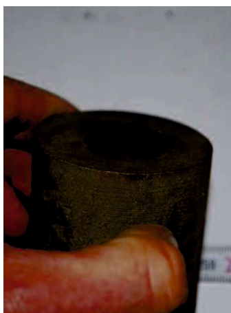
Figure 6-60: Sample So63 of Neves Corvo copper ore after 120 s of irradiation with the help of additional steel cone. Dark area and small depression at contact zone of steel cone and sample.
