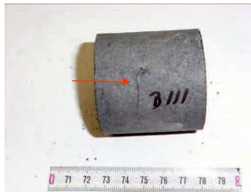
Figure 6-2: Sample B111 of Weitendorf basalt after 120 s of irradiation. Axial and radial cracks macroscopically visible (highlighted with red arrow).
