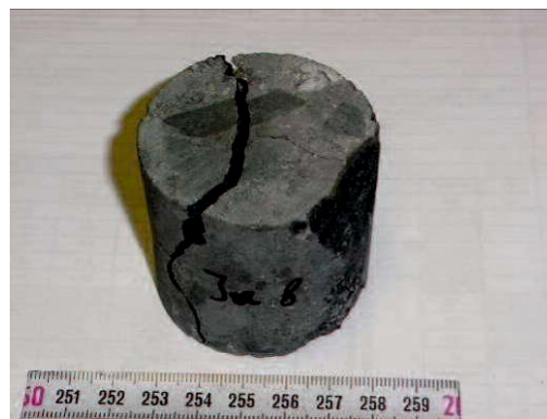
Figure 6-33: Diabase sample Ja8 after a second irradiation with microwaves for 60 s. Sample shatters along a crack.
