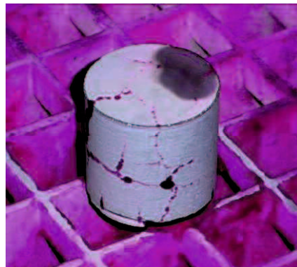
Figure 6-12: Cracked basalt sample after 120 s of irradiation. Cracks made visible with a dye-penetrant.
