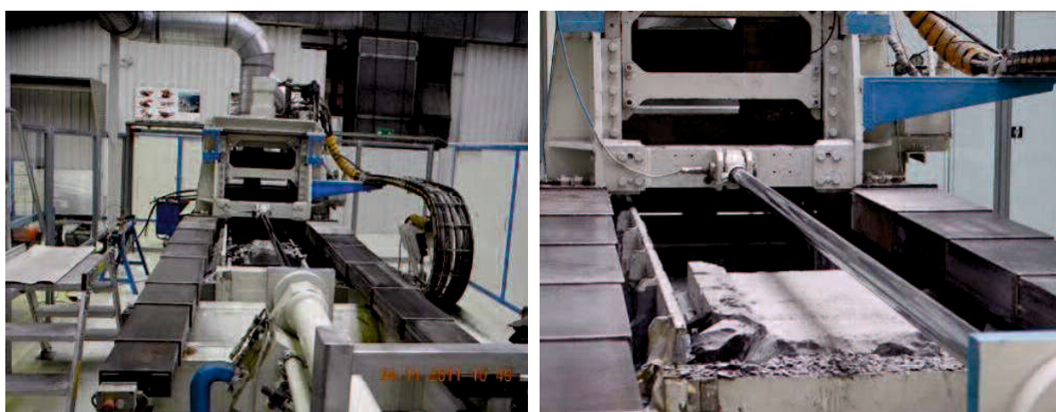
Figure 5-1: Linear cutting test rig prior to test. Sample placed in tray. The pick is dragged over the sample surface with defined speed and penetration depth.
