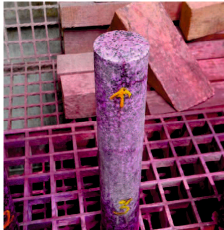
Figure 7-24: Drill core taken from granite spot irradiated for 72 s with 25 kW continuous wave. Circumferential cracks align in about 30 mm of depth.
