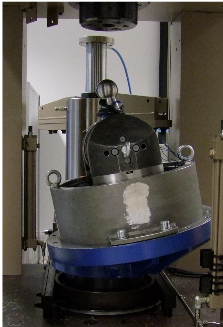
Fig. A.13.: 11° test setup with inclined clamping device
