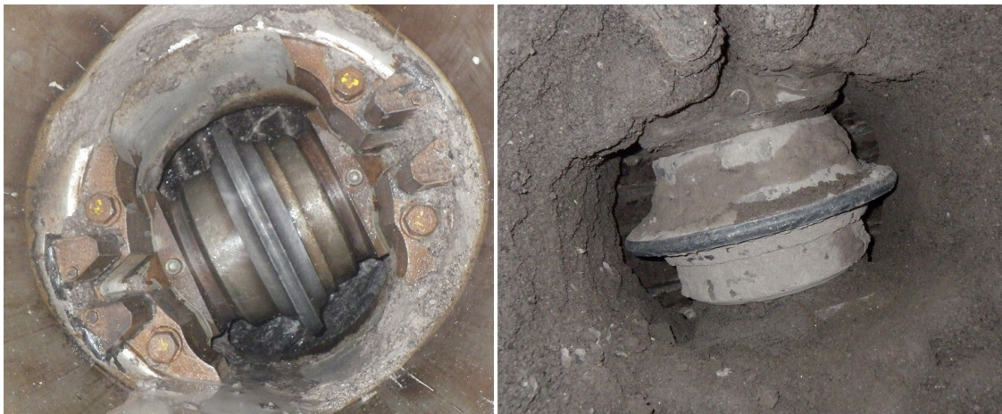
Fig. 2.1.: Inspection of sensor equipped cutters during maintenance shifts
