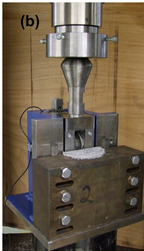
Fig. D.2.: Cut-view of the scaled rock cutting test (a), experiment setup (b)
