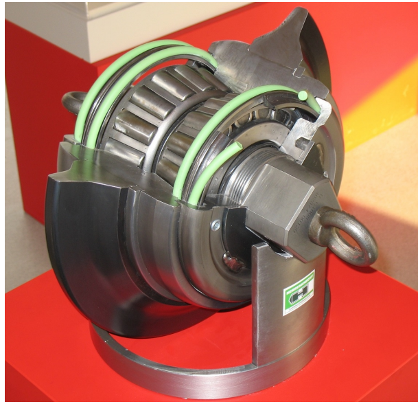
Fig. 1.2.: Cut-view of a single disc cutter (©Herrenknecht)
