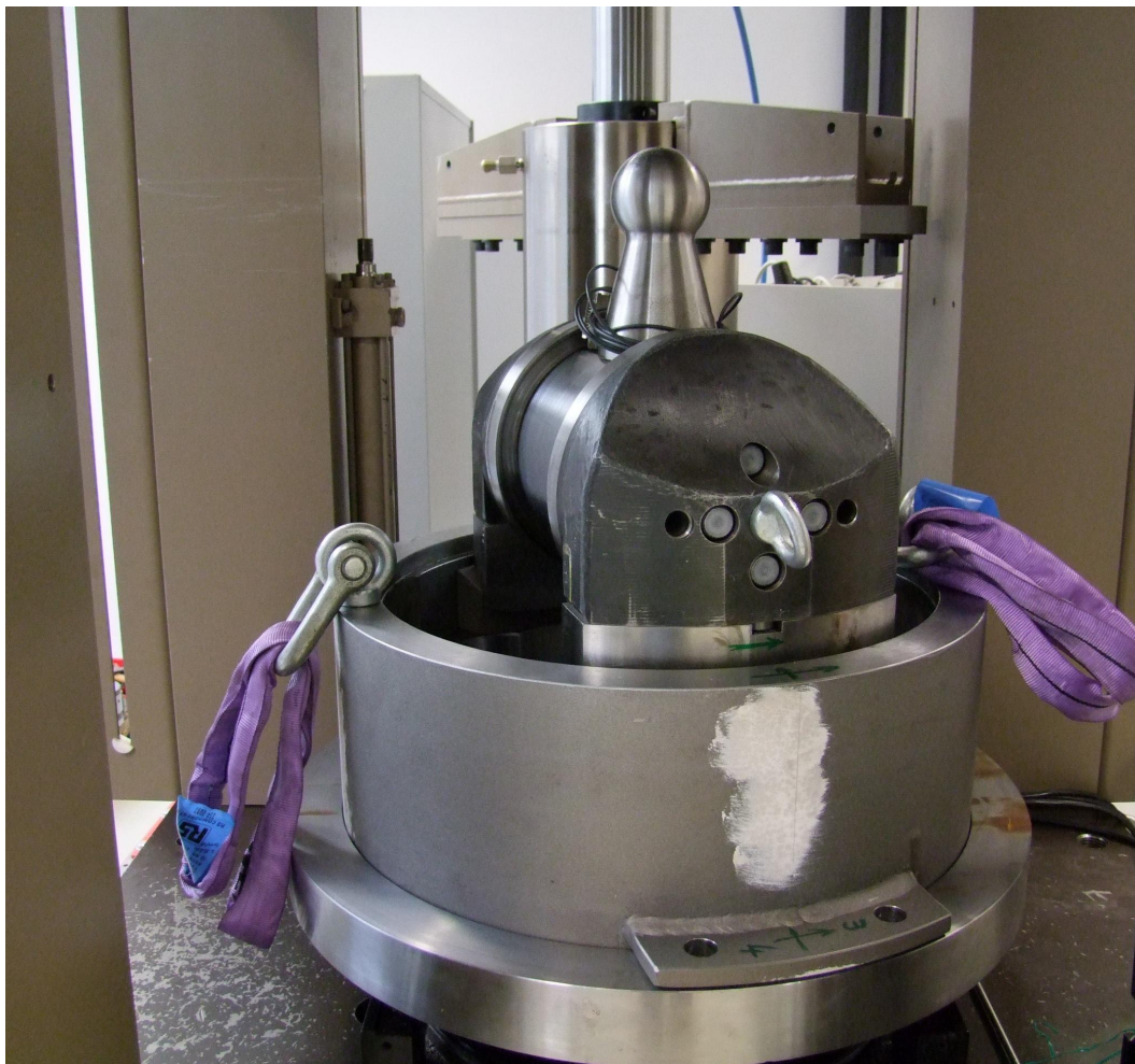
Fig. A.12.: 0^\circ test setup with flat clamping device
