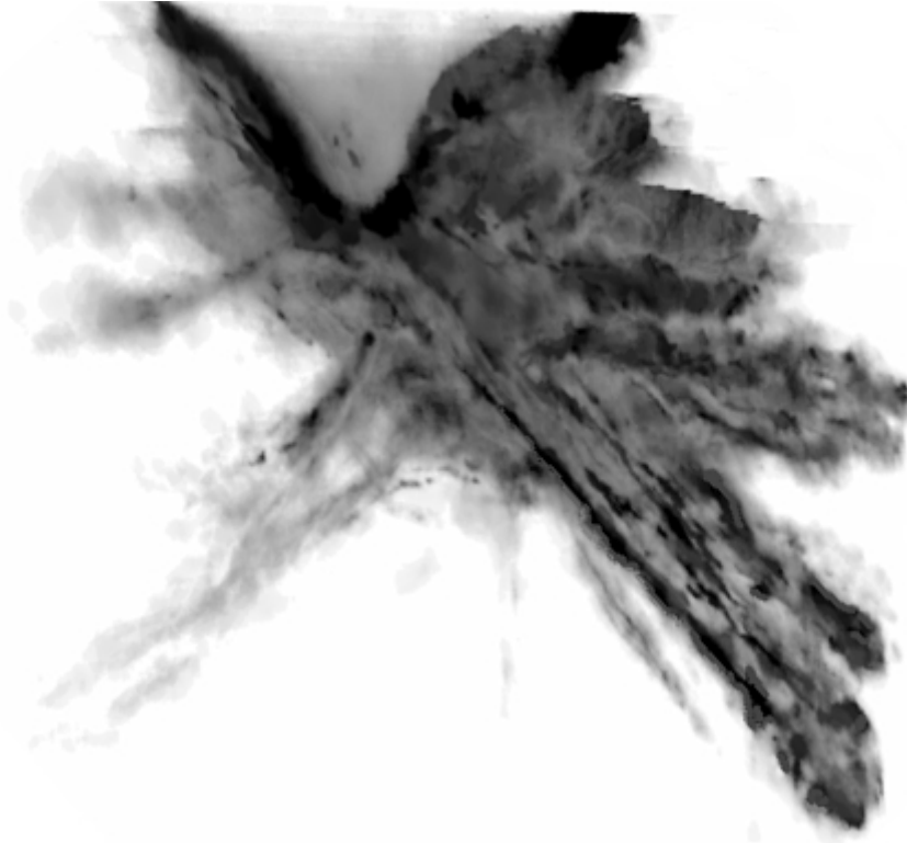
Fig. C.11.: Visualization of the crack network in an AG specimen
