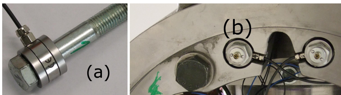
Fig. A.6.: Measurement washers (a), installation of measurement bolts (b)
