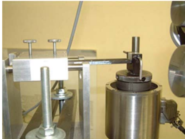
Figure 3.39 C-ELS set-up used at Laboratory B, the CFRP specimen is 150 mm long, 20 mm wide and 4.4 mm thick, in the set-up shown, the load is applied through a load-block in top of the beam which is deflected downward by the action of the test machine.
