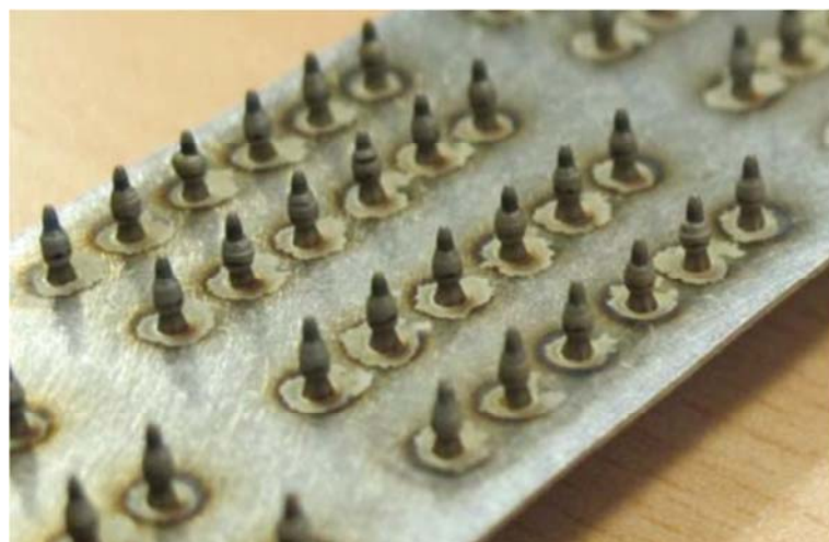
Figure 8.15: Detail of a pinned interface (pin array 1) prior to sandblasting and cleaning.
