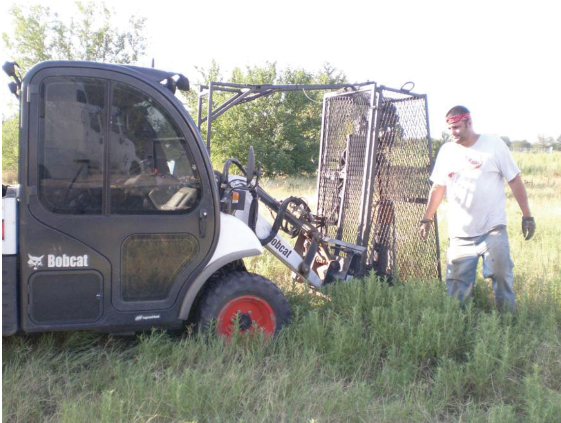
Figure 3.5 Accelerated weight drop on a tool cat, designed by the Geophysical Department of the Kansas Geological survey.
