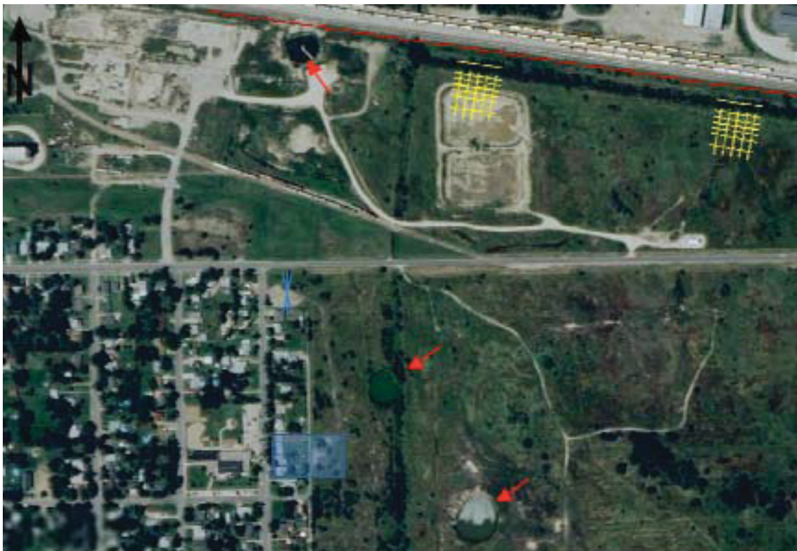
Figure 6.1 Former salt dissolution mining field in Hutchinson, Kansas. Overview of the 5 arrays (yellow, western: array 2000; yellow, eastern: array 3000; red line: array 4000; blue box: array 5000a; blue crossing lines: 5000b) deployed and recorded for this project. Three round sinkholes filled with water are recognizable in the illustration (red arrows). (From Google maps, 2011)
