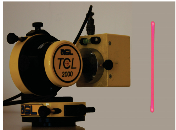
Fig. 9: The oscillating construction laser AGL TCL2000 generates a laser line of approx. 12 [mm] thickness with a frequency of 50 [Hz], i.e. one phase has a duration of 20 [ms].
