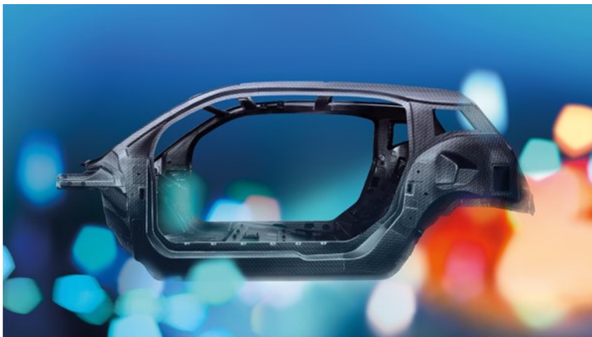
Figure 1.1: Passenger compartment of the BMW i3 made of carbon composites [11].
