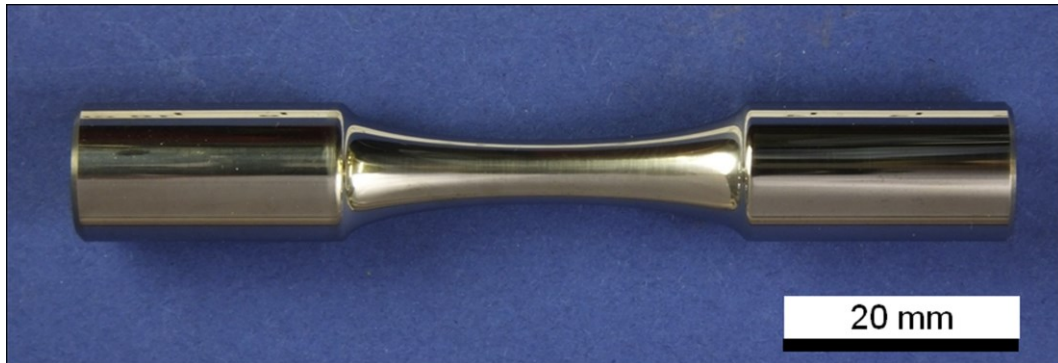
Fig.2: Specimen for uniaxial compression tests.
