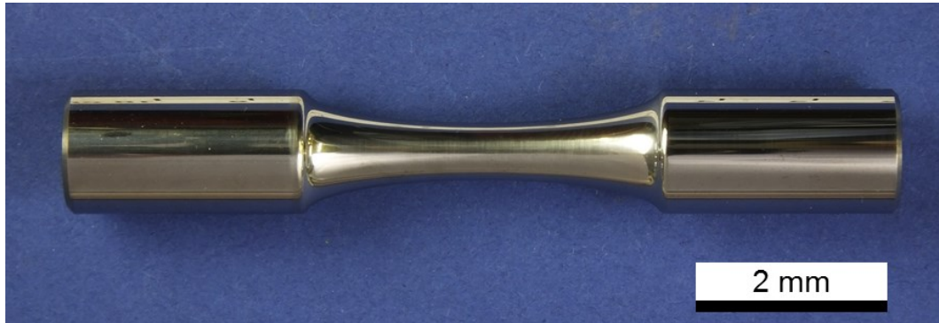
Fig. 22: Image of the uniaxial test sample shape.
