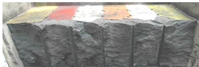
Figure 82: Front view of block #0212 after blasting of the 1 st row with 140 \mu s delay
