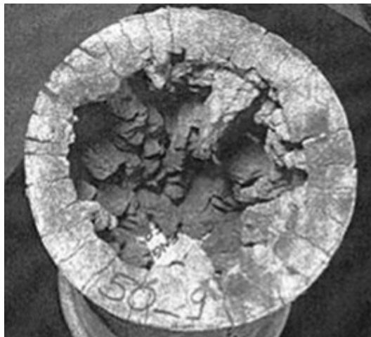
Figure 20: Crack pattern of blasted and rebuilt cylinder (Wagner, 2002)
