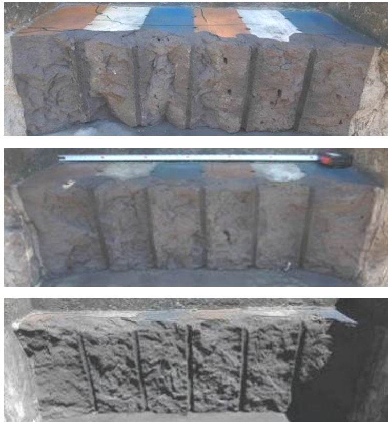
Figure 105: Front view of block #0313 after blasting of the 1 st row (top) with 140 \mu s delay, the 2 nd (middle) and 3 rd (bottom) row with 0 \mu s delay
