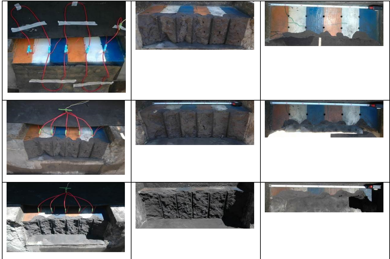
#0313: Row 1: 140 \mu s delay; Row 2: 0 \mu s delay; Row 3: 0 \mu s delay
