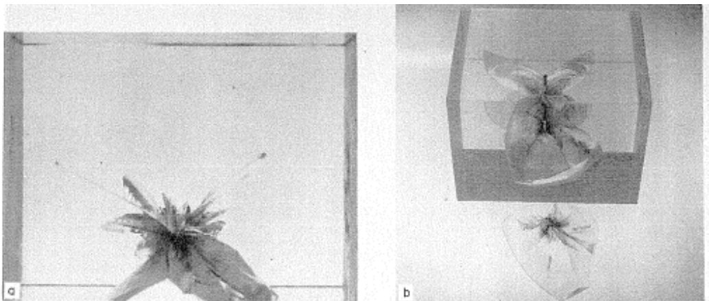
Figure 8: Top (a) and angled (b) view after blasting test (Field & Ladegaard-Pedersen, 1971)
