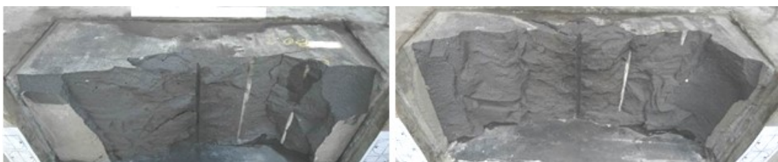
Figure 87: Front view after single-hole-shot in the middle of the 1 st (left) and 2 nd row (right)
