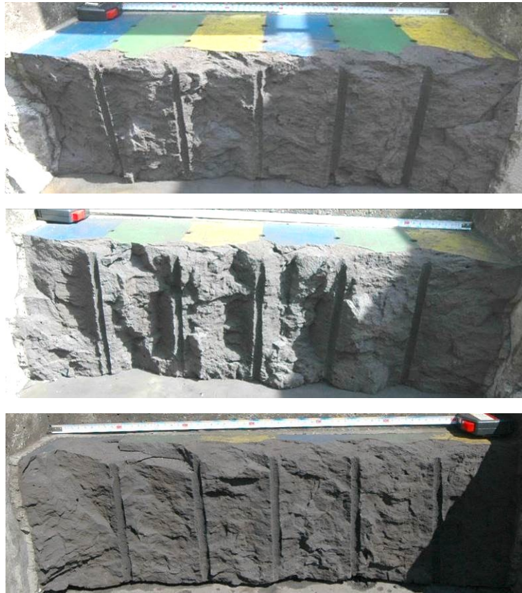
Figure 111: Front view of block #0413 after blasting of the 1 st (top), 2 nd (middle) and 3 rd (bottom) row all with 73 \mu s delay
