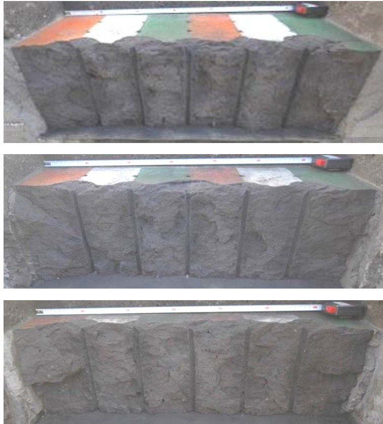
Figure 104: Front view of block #0613 after blasting of the 1 st row (top) with 28 \mu s delay, the 2 nd (middle) and 3 rd (bottom) row with 0 \mu s delay
