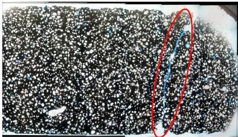
Figure 75: Example of a thin section; red ellipse marks a crack (Wrienz, 2013)
