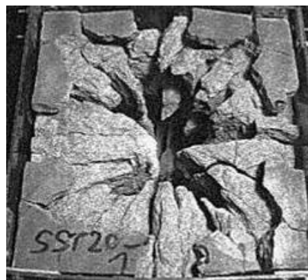
Figure 25: Crack pattern of blasted and rebuilt cube (Wagner, 2002)
