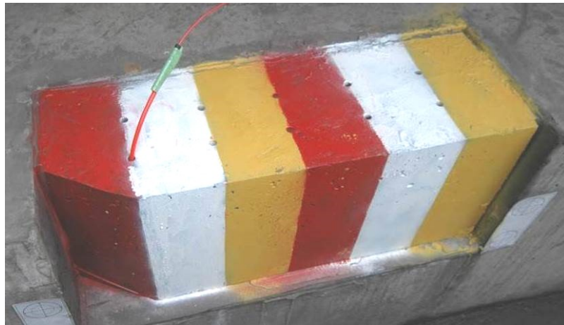
Figure 46: Test block with cut-away corner
