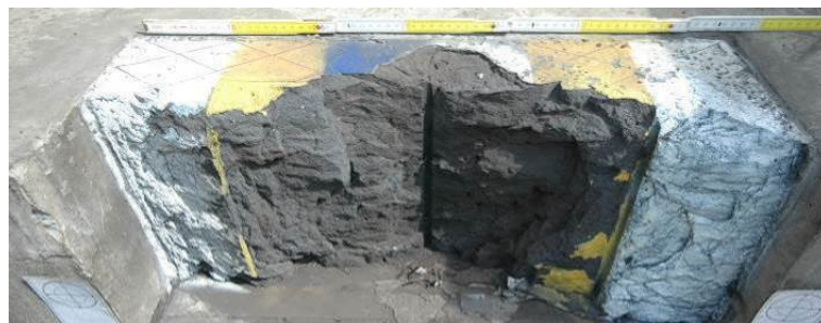
Figure 91: Front view after blasting a single hole shot in the middle of the 2 nd row
