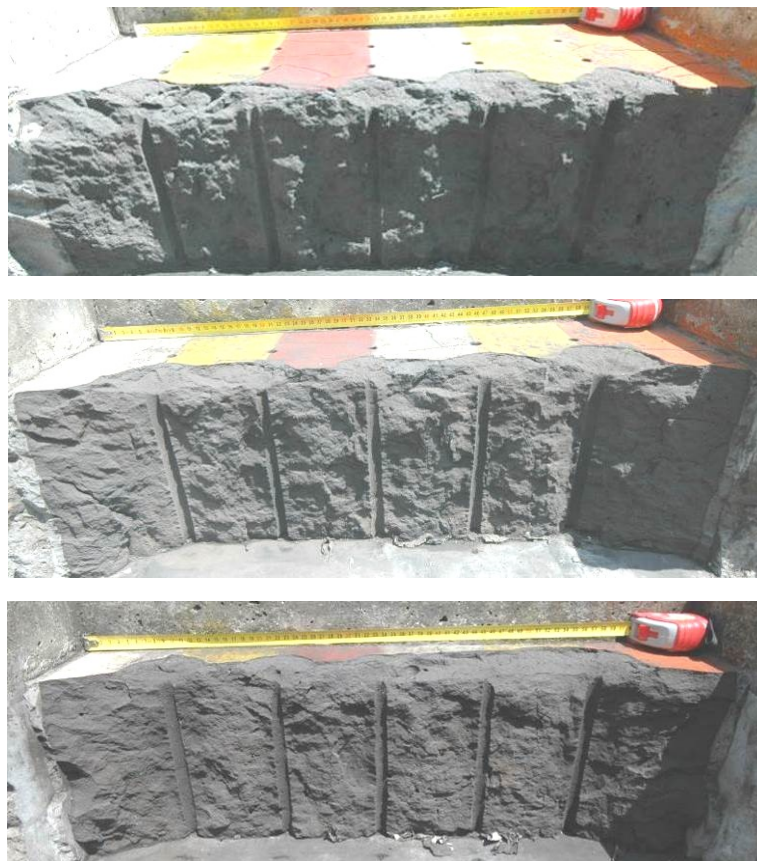
Figure 103: Front view of block #0113 after blasting of the 1 st (top), 2 nd (middle) and 3 rd (bottom) row with 0 \mu s delay
