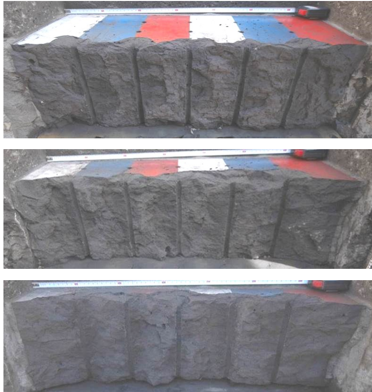
Figure 110: Front view of block #0713 after blasting of the 1 st row (top) with 28 \mu s delay, the 2 nd (middle) and 3 rd (bottom) rows with 73 \mu s delay
