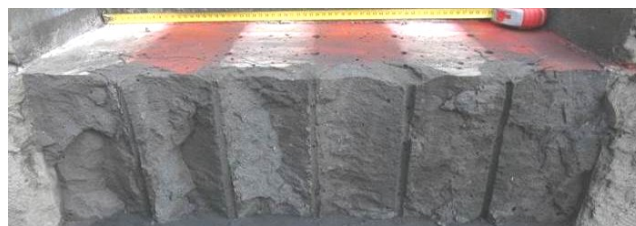
Figure 83: Front view of block #0912 after blasting of the 1 st row with 140 \mu s delay
