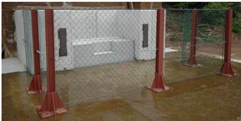
Figure 40: Yoke within the walls of the blasting site (Schimek et al., 2013). The cut-in portion in the yoke will contain the testing block
