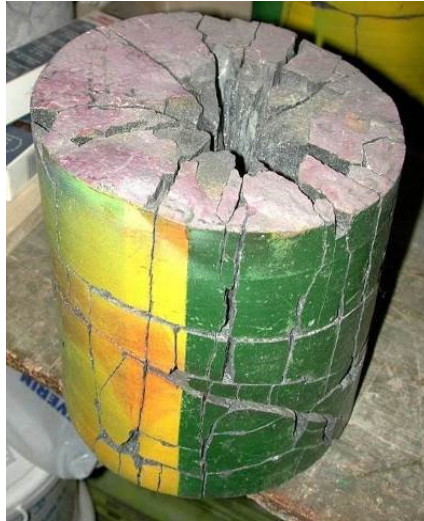
Figure 21: Vertical longitudinal cracks on the free surface of a rebuilt cylinder (Moser, 2003)
