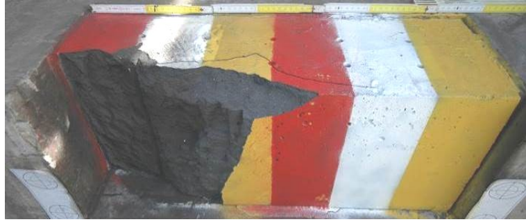
Figure 92: Testing block #0611 after blasting of the 1 st blasthole
