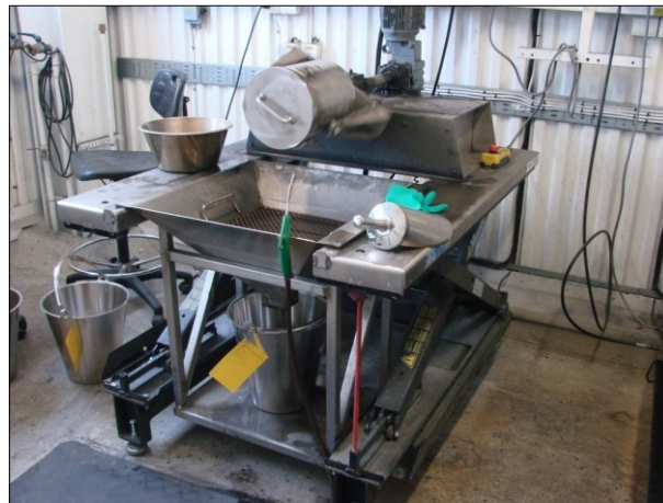
Figure 23. Laboratory tumbling mill used for the comminution tests with steel rods or steel balls as grinding media, at LKAB's mineral processing laboratory in Malmberget.
