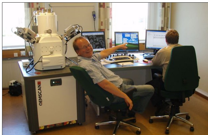
Figure 55. QEMSCAN ® E430 Pro (Carl Zeiss SEM) at LKAB's metallurgical laboratory in Luleå (Photo: LKAB).
