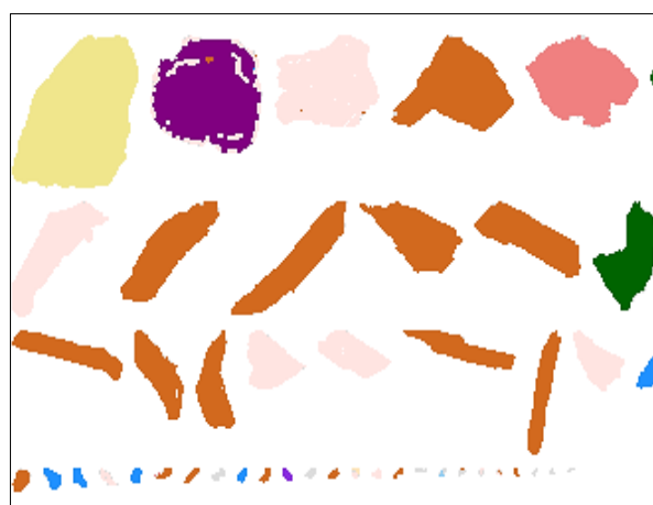
Figure 68. Fully liberated gangue minerals after crushing and comminution in a laboratory rod mill (10 minutes) and in a laboratory ball mill (35 minutes) at the laboratory of the Institute of Mineral Processing. Sample 6363, fraction 63/40 µm, mineralogy after SIP-List presented in Figure 58 A.
