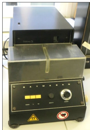
Figure 30. Satmagan by Outokumpu at the laboratory of the Institute of Mineral Processing (Photo: M. Wartbichler).
