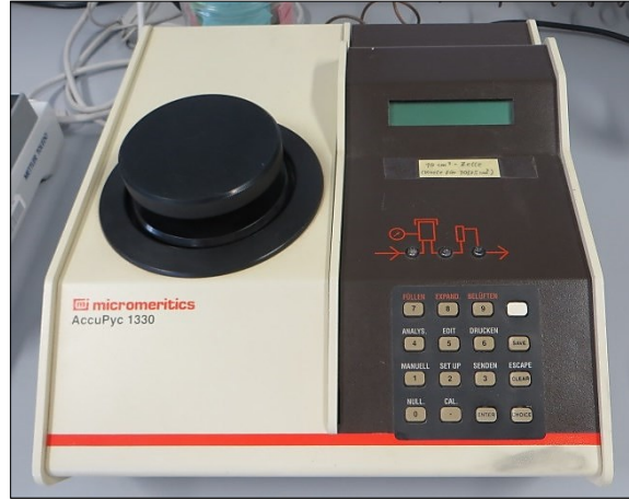
Figure 27. He-gas Pycnometer (Type AccuPyc 1330) at the laboratory of the Institute of Mineral Processing (Photo: M. Wartbichler).
