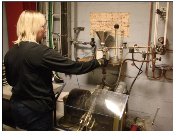
Figure 26. Apparatus for the Davis magnetic tube tests at LKAB's mineral processing laboratory in Malmberget.
