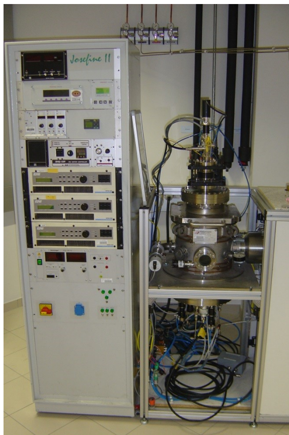
Figure 17: Laboratory-scale magnetron sputtering system “Josefine II” used to synthesize the TiN/Cu layer stacks discussed in chapters 3 and 4.
