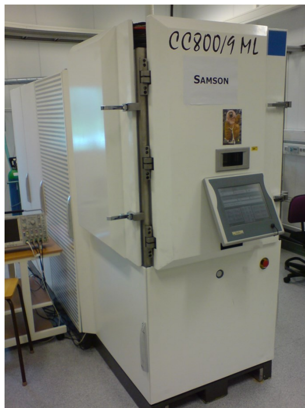
Figure 18: Industrial-scale CemeCon magnetron sputtering system “Samson” used to synthesize the TiN/Cu and TiTaN/Cu layer stacks discussed in chapters 5 and 6, respectively.
