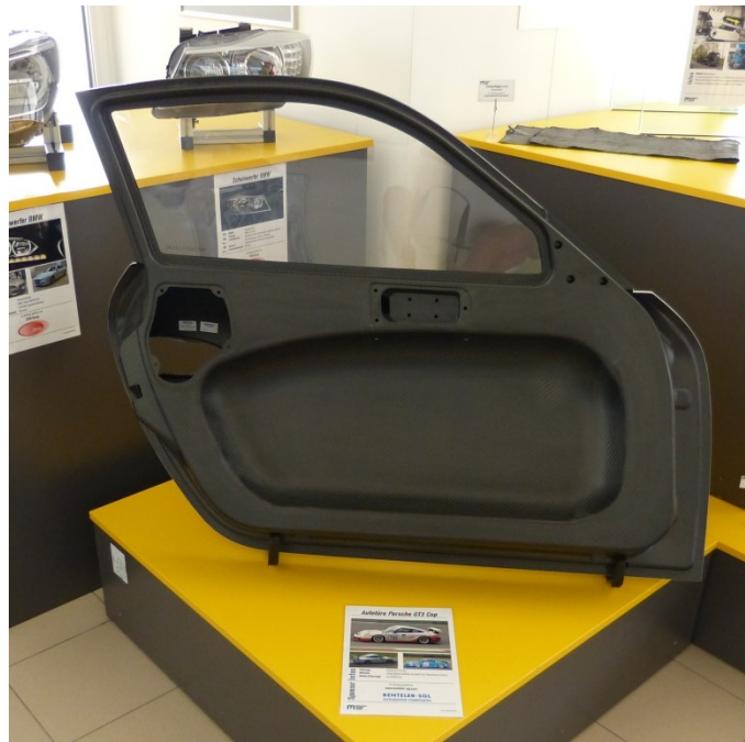
Figure 2-1: Car body parts made of carbon composites.
