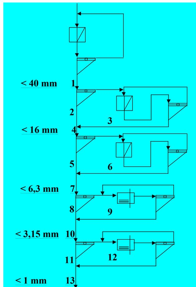
**Figure 4: Flowsheet of the Optimized Comminution Sequence built up for the Less Fines Project**
