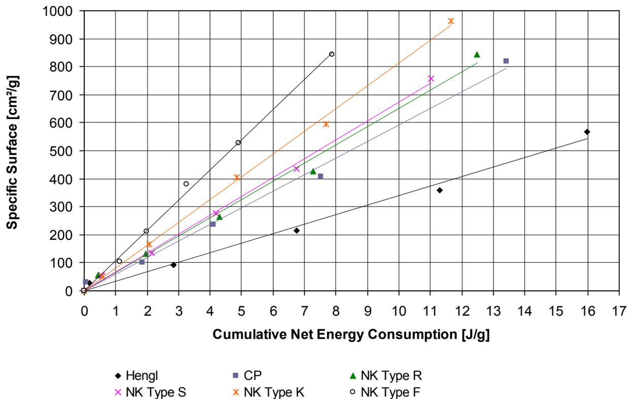
**Figure 20: Energy register functions of the six rock samples: amphibolite Hengl (Hengl), limestone Cementos Portland (CP), limestone Nordkalk (NK) types R, S, K, and F**
