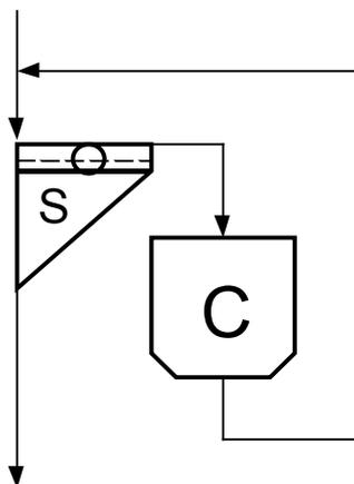
**Figure 1: Scheme of the closed circuit design with prescreening.**
