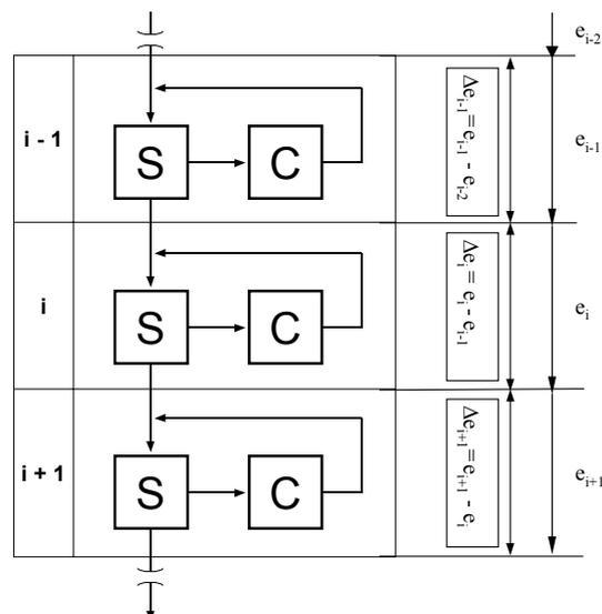
**Figure 2: General representation of the principle of energy optimized comminution according to Steiner [2]**
