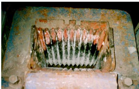
**Figure 6: View into the mouth, both jaws are grooved down to the discharge**
