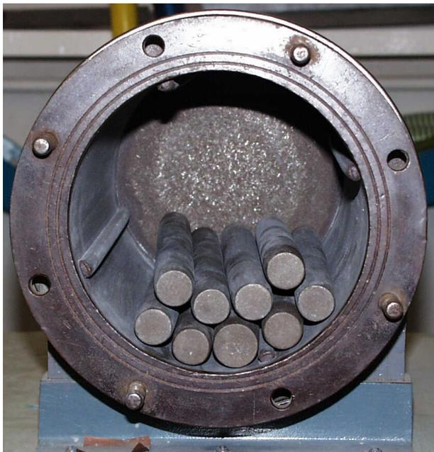
Figure 12: View into the mill
