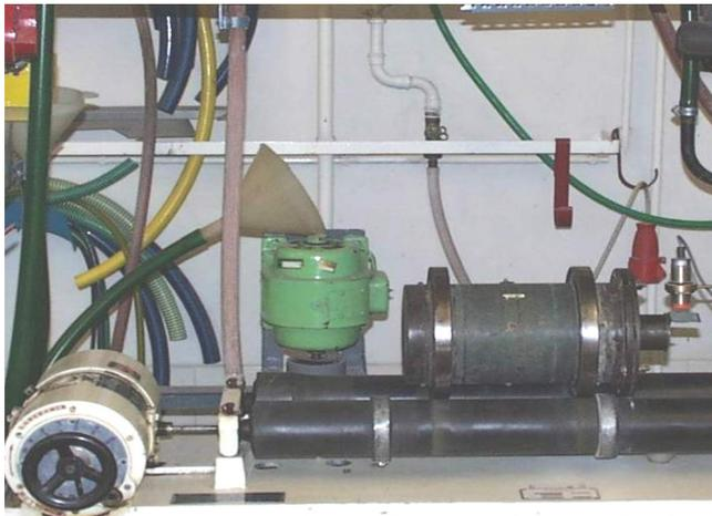
Figure 11: Test rig of the rod mill consisting of the roller drive, the rod mill and the revolution counter
