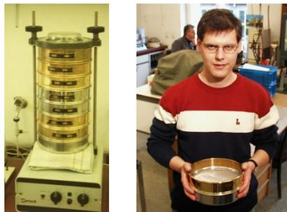
**Figure 17: Prescreening on a test sieve shaker, completed by manual screening**
