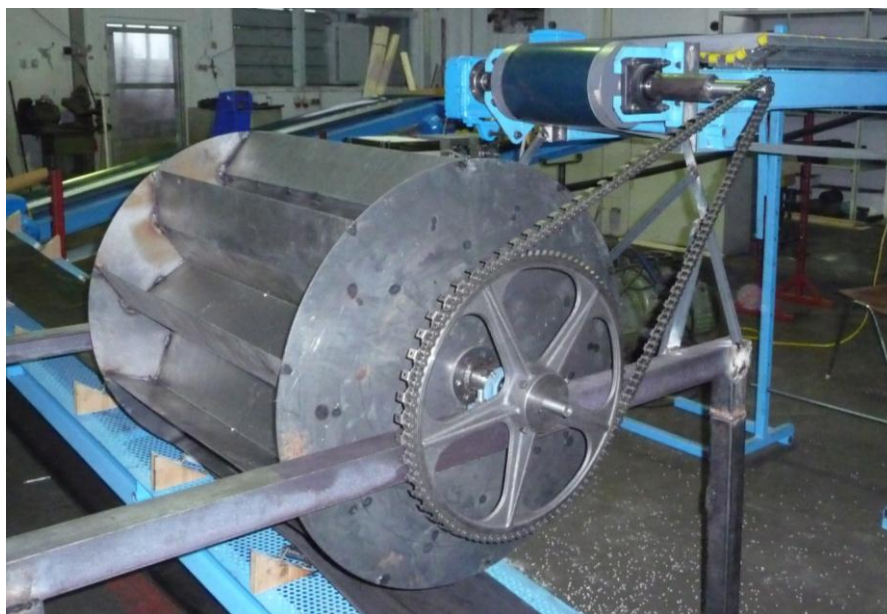
Figure 4: Prototype of a simple "Solid State Material Driven Turbine"
