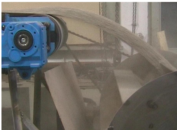
Figure 5: "Solid State Material Driven Turbine" in operation
