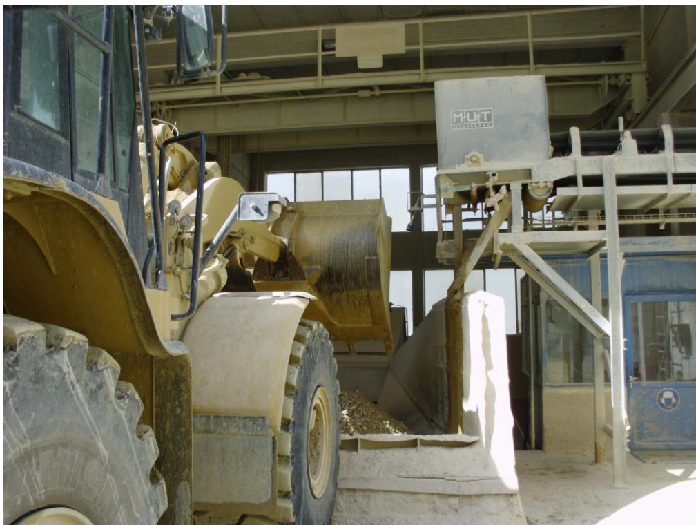
Figure 15: Wheel loader for feeding the crusher
