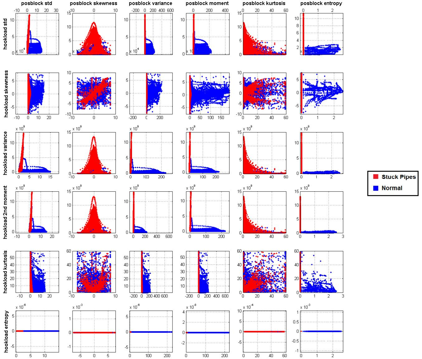
Figure 2: scatter plots of key statistical features selected by the experts as relevant for identifying “stuck pipes” problems.
