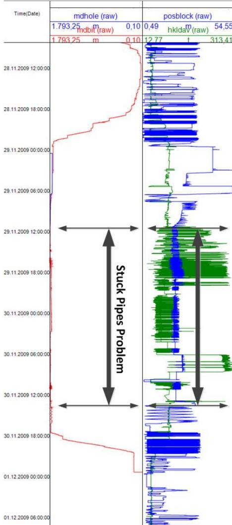
Figure 1. Identifying “Stuck Pipes” problem on a time chart of drilling sensor data
