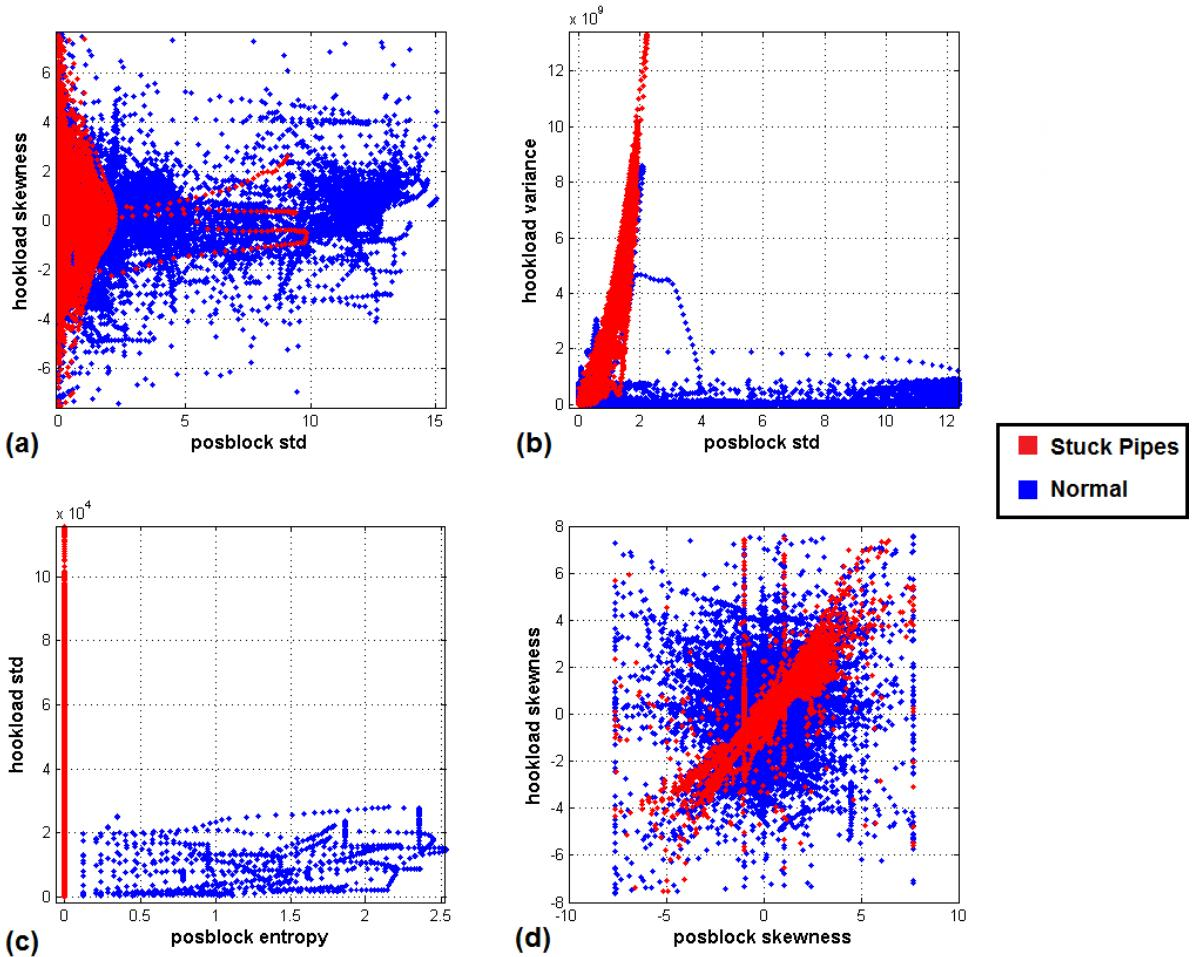
Figure 3. Detail scatter plots views that identify the “stuck pipe” problems. (a, b) different but overlapping distributions for the two classes. (c) the posblock entropy as discriminative but unreliable feature (d) the skewness features exhibit noticeable difference in the trends.
