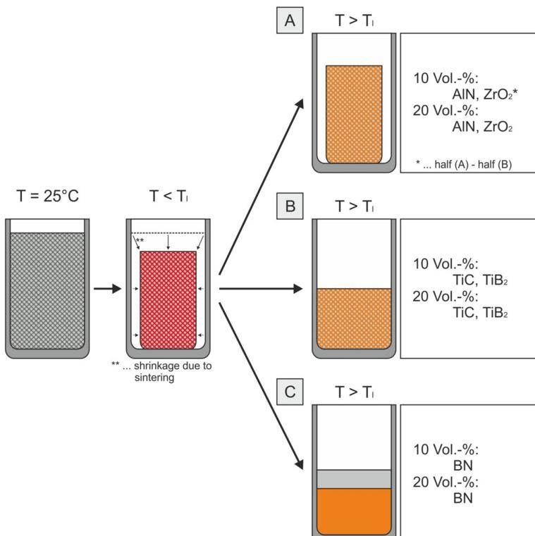
MMC keeps sintered geometry
