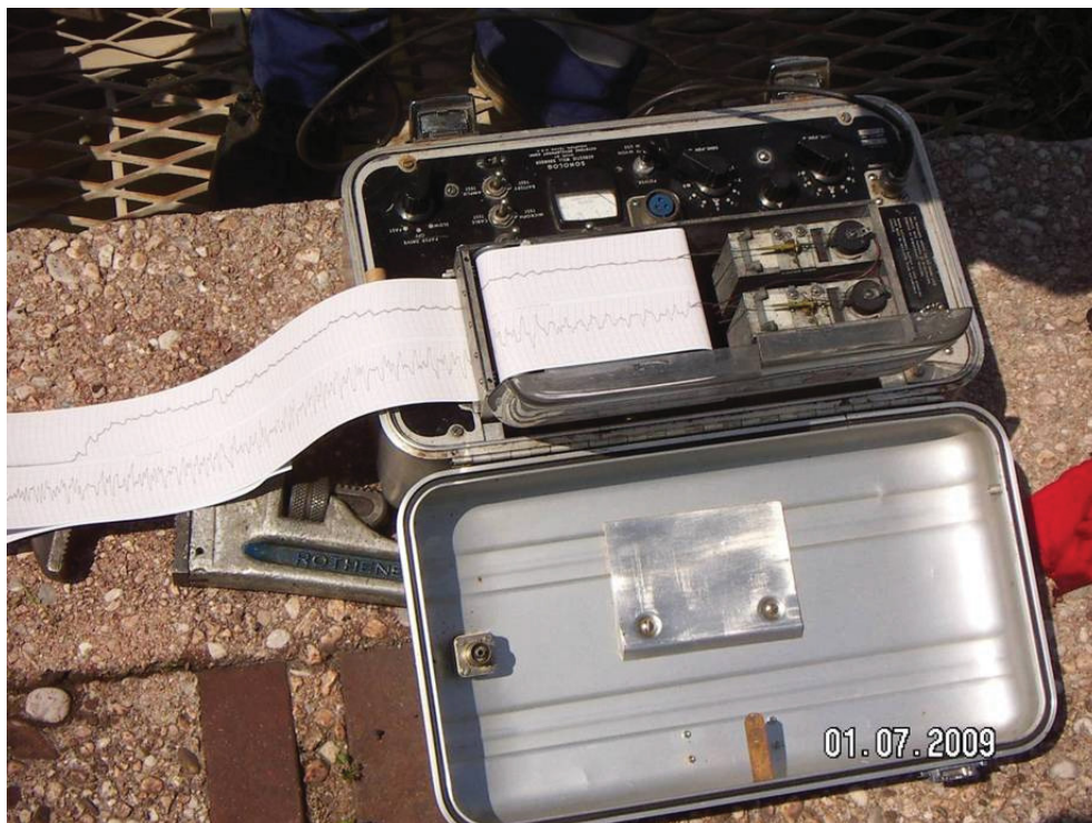
Fig. 2 – The Rectifier and Printer of the Conventional Fluid Level Measurement Tool. Each reflection caused at a tubing connection and at the fluid level itself is recorded and printed for further analysis.
