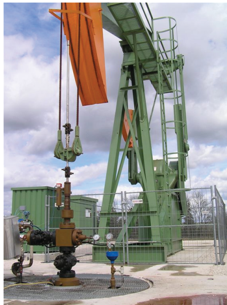
Fig. 10 – Fluid level Measurement Tool mounted on a sucker rod pumped well BH-009.
