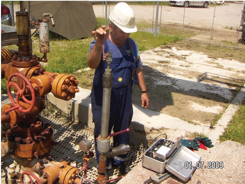
Fig. 1 – Conventional Fluid Level Measurement Tool – Casinggas is vented shortly to the atmosphere and closed suddenly. Noise is induced.
